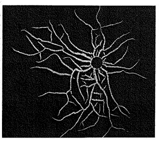
"This...is the self registered picture of a dielectric in the process of breakdown. The mathematics of breakdown is as important as it is unfamiliar even to the average physicist. It is closely allied to the mathematics of crackle finish... The significance of the processes of breakdown is great not only in physics, but even in the study of sociological processes."
