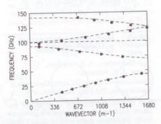
QWE4 Fig. 2. Photonic band structure of a two-dimensional array of alumina cylinders with the electric field parallel to the rod axes. Dots are the experimental points; lines are theoretical prediction.
