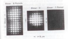
QWE3 Fig. 3. Images of lattice and unit cells obtained with a shearing interferometer for shears of (a) 6 lattice periods, (b) 0 lattice periods, (c) 1 lattice period.
