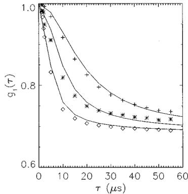
Fig. 12. Experimental measurements of the normalized temporal field correlation function for three different flow speeds in comparison with theory. Measurements for flow speeds of 0.442, 0.884, and  $1.77 \text{ cm s}^{-1}$  are indicated by the symbols +, \*, and  $\diamond$ , respectively. The curves, from top to bottom, are calculated with the experimental parameters given in Fig. 11 and with effective shear rates of 3.0, 6.0, and  $12.0 \text{ s}^{-1}$ , respectively.
